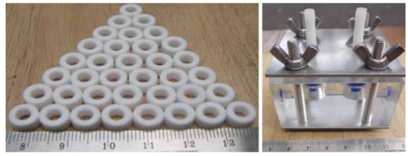
9. Designed and completed the machining of perfusion chamber unit to DTERT lab.
