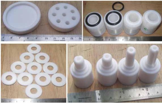
8. Completed the machining of different Teflon moulds, sample preparation rings and Teflon plug to TEM, TIC and MPL lab.
