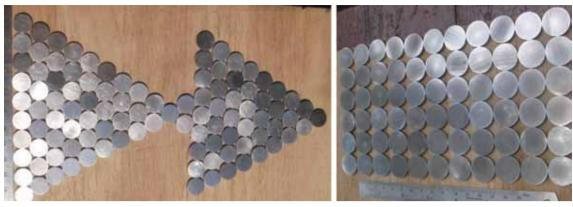
7. Completed the machining of different size blanks for testing the coating to CCF lab.
