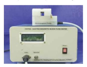
The prototype was tested on an extracorporeal circuit with blood analogous fluid as the medium and actual flow rates versus displayed flow rate on the prototype were studied. Results showed that the prototype developed has accuracy more than 95% and has very less signal rift and instability issues.
