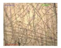
Optical Microscopic Imaging of Electrospun Terpolymer Fibers
