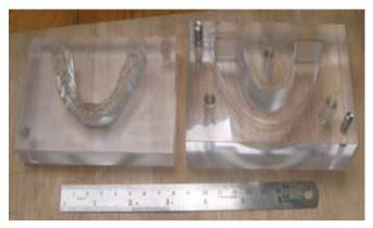
4. Completed the machining of Needle penetration test setup fixture to DTL to study the penetration forces on graft materials
